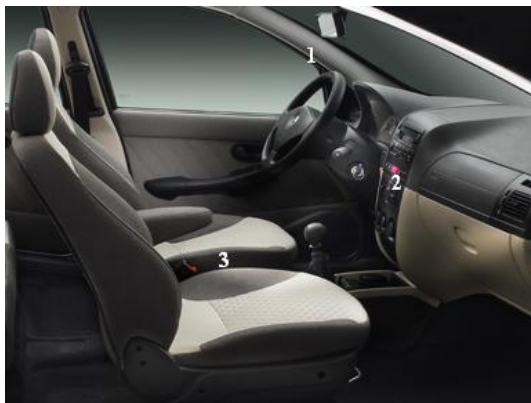
Figure 1. Experimental setup inside the cabin, 1-Temperature, Rh probe, 2-Air velocity, 3-Data logger.
